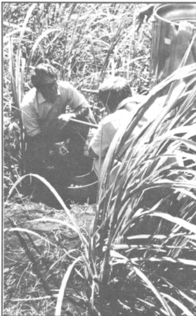
Hydrologic characteristics of soils under different land uses were studied by comparing rates of water percolation in sugar cane field with those under under forest cover.
